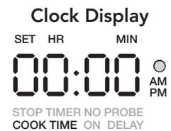
2. Toggle "SELECTOR KNOB" right to increase or left to decrease to set desired time. Time will scroll in one minute increments per individual toggle. If "SELECTOR KNOB" is held in either right or left position, time will increase or decrease in 10 minute increments until desired time is reached.
